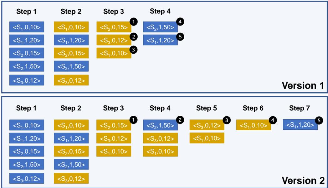
Fig. 5. The two versions of the gas price ranking method implemented in Geth during the Byzantium period. They differ in how the *nonce* parameter is dealt with.
