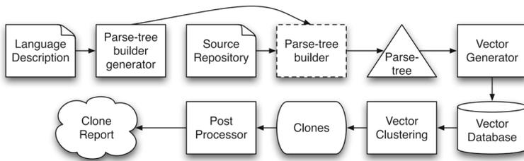
**Fig. 4** Deckard's architecture Jiang et al. (2007a)
