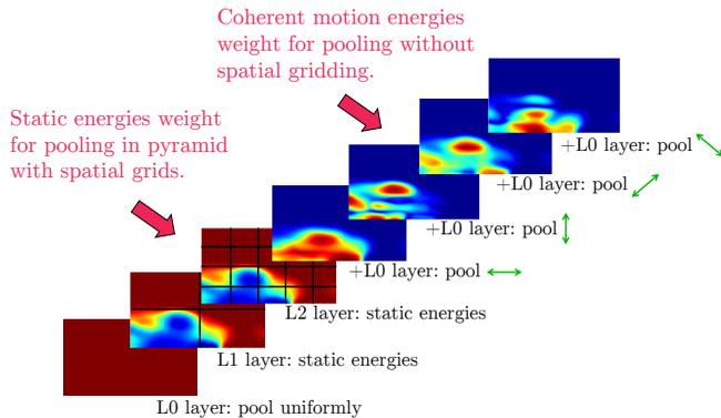
Fig. 5: Dynamic Spacetime Pyramid. Larger responses (hotter colors) in the static energies guide pooling into coarse (L0) as well as fine grids (L1 and L2). In contrast, coherent motion energies limit pooling to the coarsest grid only (L0). Green arrows along the sides of the coherent motion plots indicate directional tunings. Input imagery is from the Street Sequence, as shown in Fig. 4.
