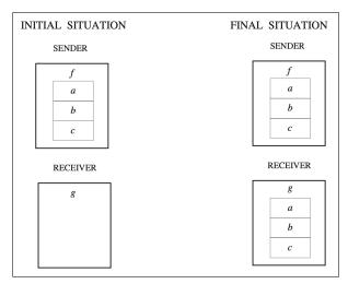
Consider the initial model  $(m_0)$  for the above system which only addresses the above **REQ1**: a file is transmitted from the sender to the receiver.
