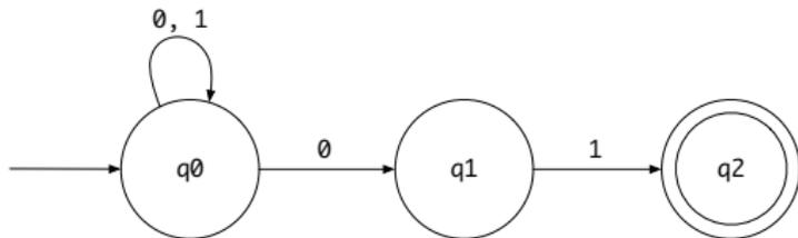
**Subset construction** (with *lazy evaluation*) produces a **DFA** with  $\delta$  as:
