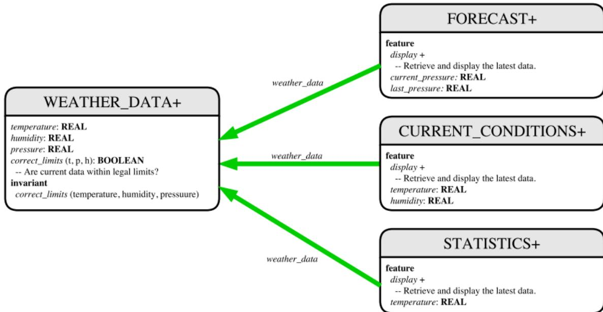
**Whenever** the `display` feature is called, **retrieve** the current values of temperature, humidity, and/or pressure via the `weather_data` reference.
