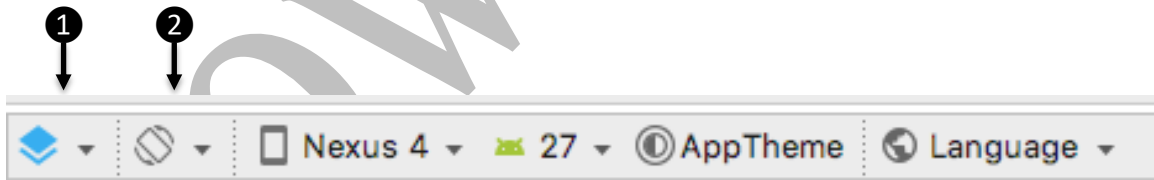
Figure D0.1 Configuring the design editor: ❶ choose the design surface, ❷ choose the device orientation.
