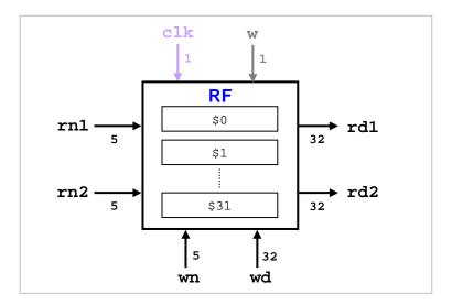
In order to read the contents of two registers, we supply their register numbers thru rn1 and rn2 (5 bits each). After some delay, the corresponding contents of these two registers will become stable on rd1 and rd2. In order to store a 32-bit value in some register, we supply it on wd and supply the 5-bit register number on wn. The value will be written on the positive edge of clk if and only if w=1. Hence, w is in fact an enabler. Note that register \$0 is read-only and its value is 0.
