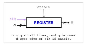
As all sequential components, a register has an internal state, denoted by q, and it is made up of n bits, where n is a parameter set upon instantiation. The output z is equal to q at all times; i.e. you can always read the content of a register. In order to write (i.e. store) a value in the register, supply the value through d, set enable to 1, and then wait until the clk input rises from 0 to 1.
