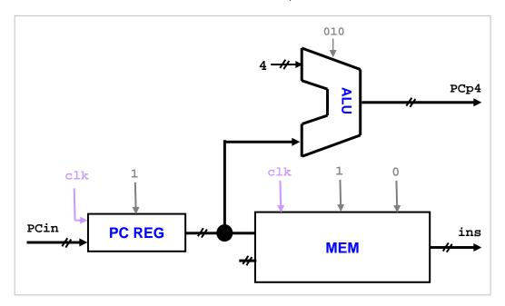
We connect the output of the PC register to the address input port of our mem unit. Since we always read instructions from memory and never write, the memIn port of mem is left unconnected and the signals memRead and memWrite are set to 1 and 0 respectively. Argue that the clk input of mem is irrelevant and can be left dangling.
