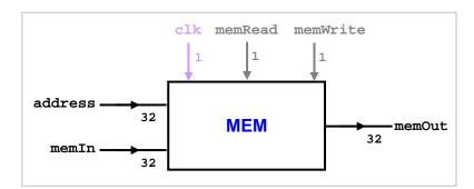
This sequential component is made up of many 32-bit words. In order to read a word, set its address on address and set memRead. After some delay, the word's content will become stable on memOut. To write, set the data to be written on memIn, set the destination address on address, and set memWrite. The data will be written on the destination at the next positive edge of clk.
