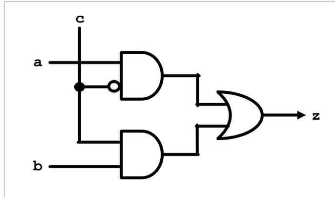
Note that the circuit has three 1-bit inputs and one 1-bit output.
