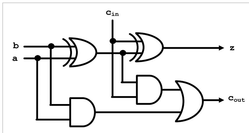
Note that the circuit has three 1-bit inputs and two 1-bit outputs. It is made up of two **xor** gates, two **and** gates, and an **or** gate.
