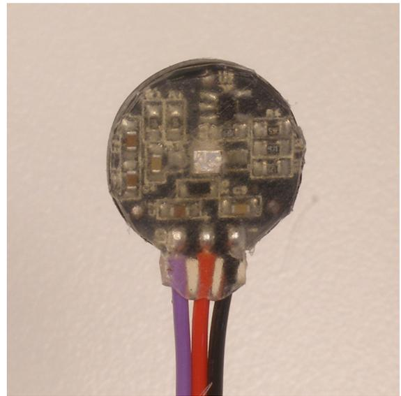
This is the basic Pulse Sensor Hot Glue Seal, It's also got the clear vinyl sticker on the front face. We're calling this 'Water Resistant', ready to be handled and passed around from fingers to earlobes or whatever. It is not advised to submerge or soak the Pulse Sensor with this basic seal. Now you can stick on the velcro dot (included) and make a finger strap with the velcro tape (included)!
