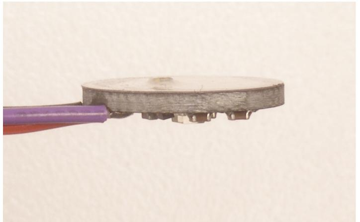
When you are happy with the way it's lined up, squeeze it onto the face all at once! The sticker (made of vinyl) will kind of stretch over the sensor and give it a nice close fit. If you get a wrinkle, don't worry, just press it down really hard and it should stick. We gave you 4, so you can replace it if necessary.
