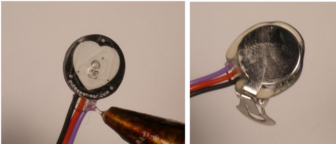
Allow the hot glue to ooze out around the ear clip. That will ensure good coverage. Take care not to let the hot glue cover around the ear clip hinge, as that could get in the way of it working. Trimming is easy with nail clippers (as above) or your trimming tool of choice. Don't trim the wires by mistake!!!
