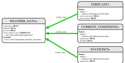
Whenever the display feature is called, retrieve the current values of temperature, humidity, and/or pressure via the weather\_data reference.
