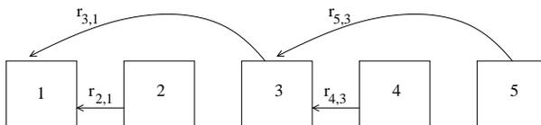
Fig. 2. An Example of DAG Source Model for H.264/AVC Video with Reference Frame Selection
