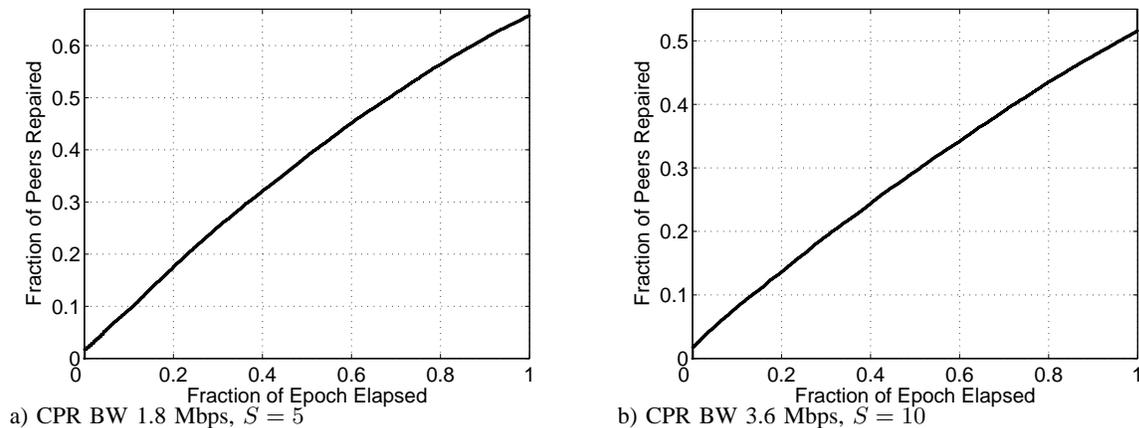
Fig. 6. CDF of the number of peers repaired during one epoch time.
