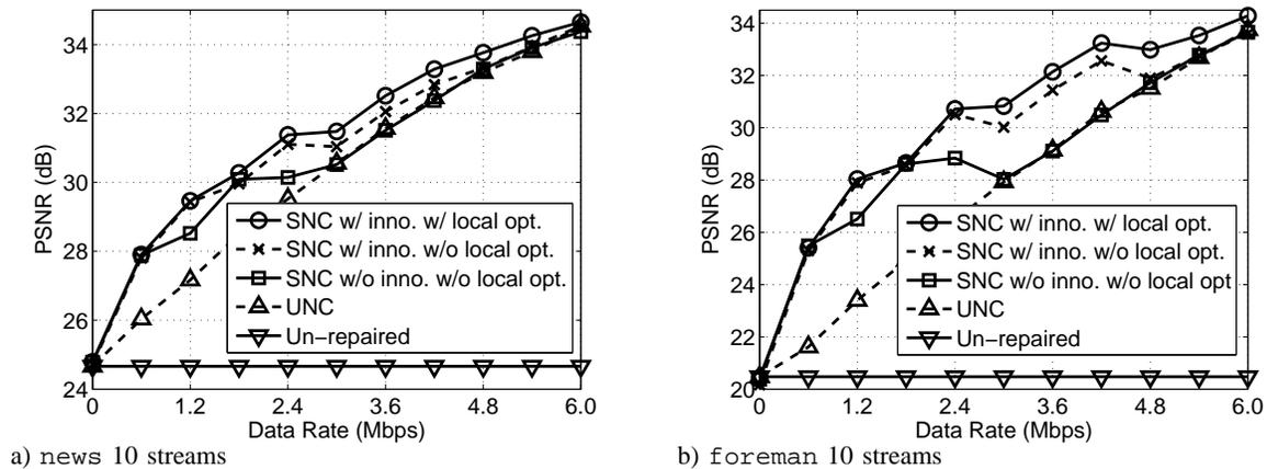
Fig. 8. PSNR for the news and foreman sequences under various CPR transmission rates and SNC scheme settings.
