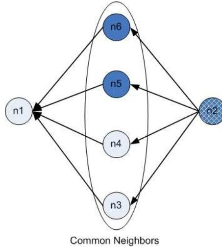
Fig. 4. Common neighbors in CPR network.  $n_3, n_4, n_5$  and  $n_6$  are common neighbors of  $n_1$  and  $n_2$ .  $n_1, n_3$  and  $n_4$  watches  $s^1$ ,  $n_2, n_5$  and  $n_6$  watches  $s^2$ .  $n_2$  receives one packet of  $s^1$  during the repair process.
