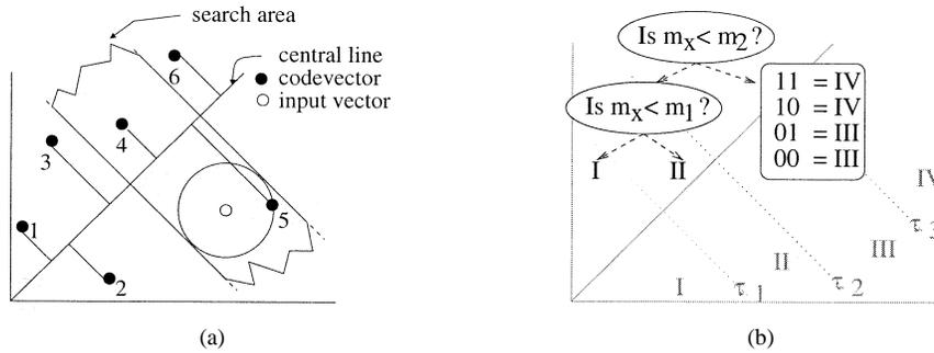
Fig. 8. (a) Equal-average VQ encoding and (b) hybrid encoding implementation.
