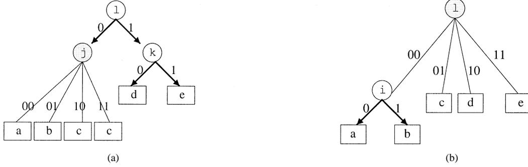
Fig. 5. Examples of prefix decoding using 1-bit logic and table lookup. (a) Prefix decoding configuration 1 and (b) prefix decoding configuration 2.
