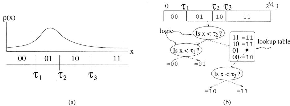
Fig. 6. (a) Nonuniform SQ and (b) hybrid encoding implementation.
