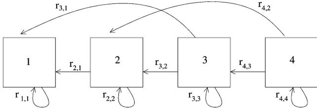
Fig. 2. DAG source model. The quantities  $r_{3,3}$ ,  $r_{3,2}$ ,  $r_{3,1}$  represent, respectively, the number of bytes for three different choices of coding frame 3, namely, intra-coding, P-frame with frame 2 as reference and P-frame with frame 1 as reference.
