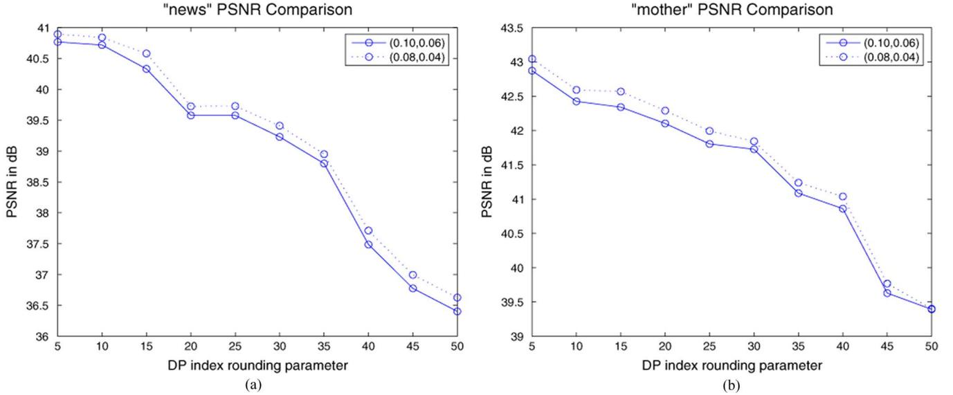
Fig. 12. Visual quality degradation of *news* and *mother* as index rounding parameter ( $K_{\text{IR}}$ ) increases. (a) PSNR for *news*. (b) PSNR for *mother*.
