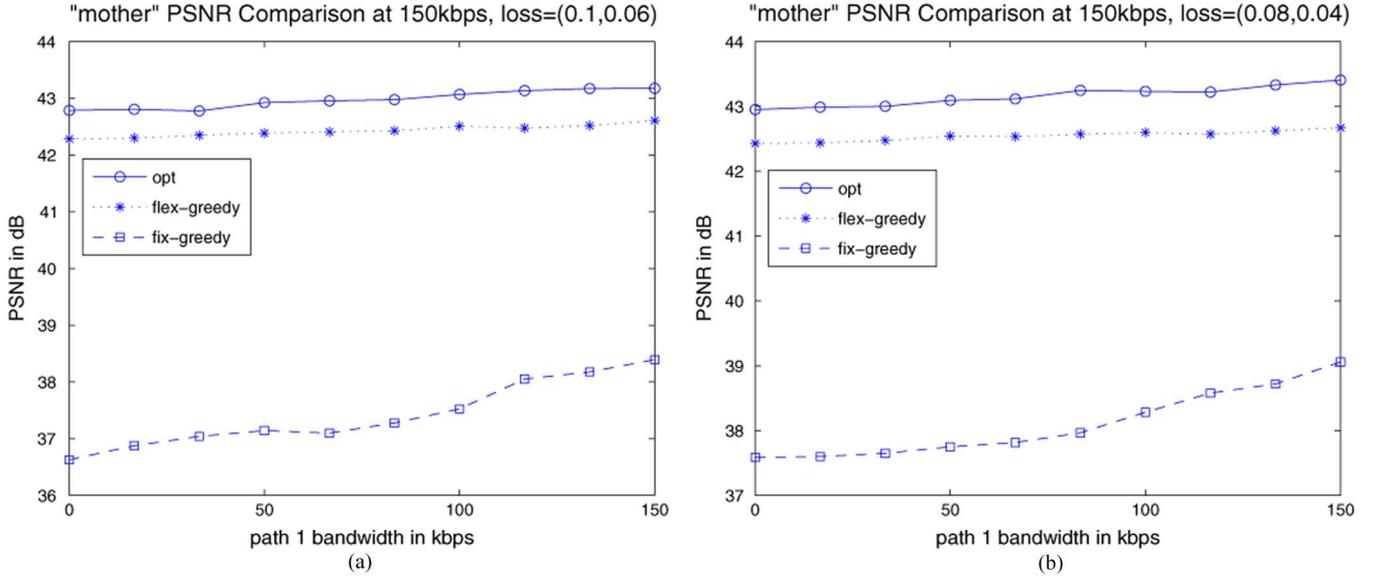
Fig. 10. Streaming performance for *mother* in PSNR for varying path-1 bandwidth for fixed total bandwidth = 150 kbps. (a) loss rate = (0.10, 0.06). (b) loss rate = (0.08, 0.04)
