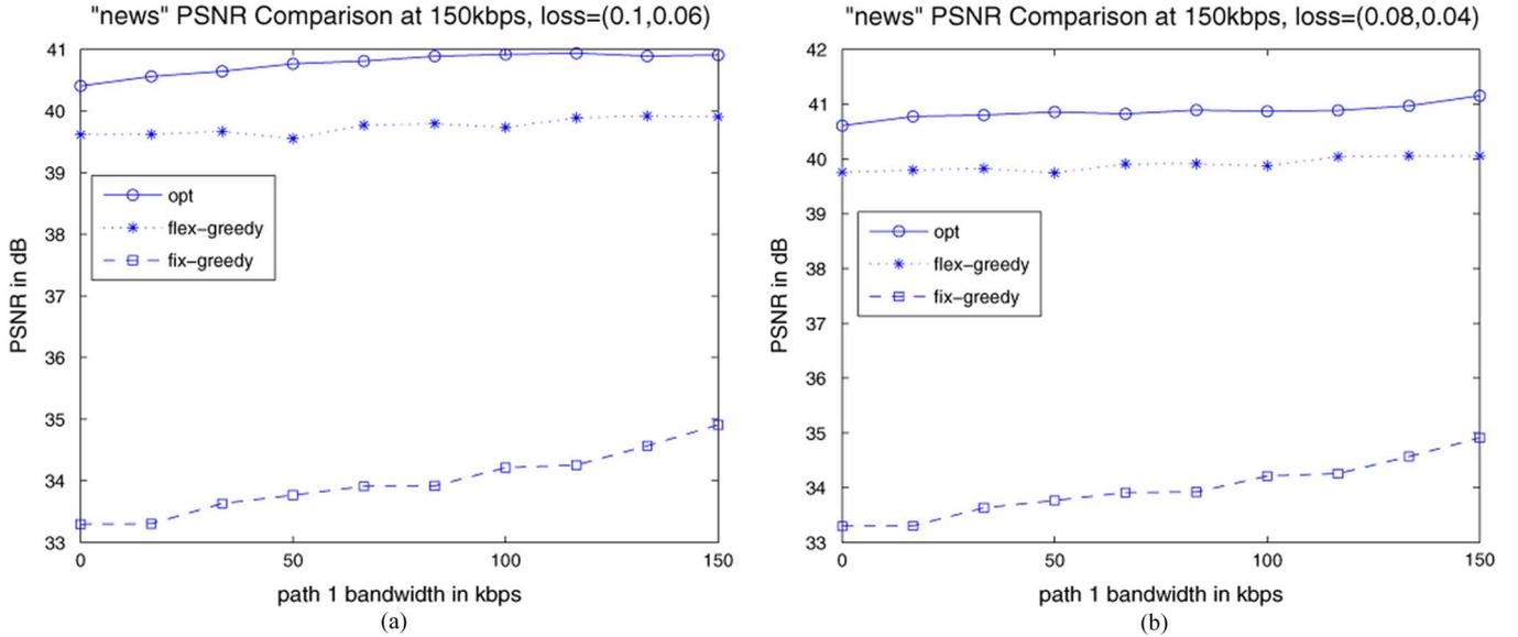
Fig. 9. Streaming performance for news in PSNR for varying path-1 bandwidth for fixed total bandwidth = 150 kbps. (a) loss rate = (0.10, 0.06). (b) loss rate = (0.08, 0.04).
