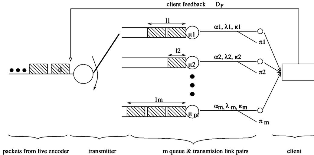
Fig. 8. Network simulator muns is used to simulate queuing, transmission, and losses of packets.
