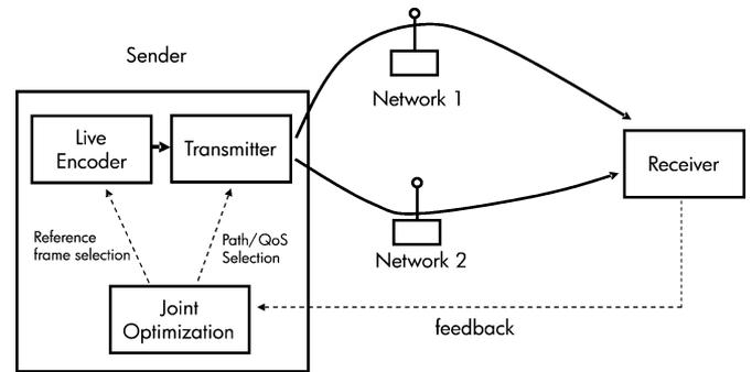
Fig. 1. Application scenario of interest involves live streaming with feedbacks over multiple network interfaces. The sender is responsible for jointly selecting the reference frames and associated QoS levels on multiple transmission paths. An effective scheme to realize such joint optimization is the focus of this paper.
