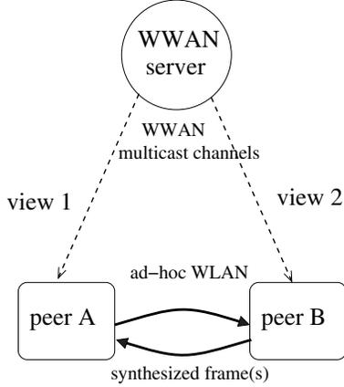
**Fig. 1.** System Model for Multiview Video Streaming
