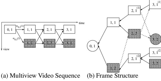
**Fig. 3.** Example of Redundant Frame Structure. I- and P-frames are drawn as circles and boxes, respectively. A solid edge from  $F_{i+1,k}$  to  $F_{i,j}$  in (b) means a P-frame  $F_{i+1,k}$  is predictively coded using reference frame  $F_{i,j}$ . A dotted edge from  $F_{i,j}$  to  $F_{i+1,k}$  in (b) means a schedule  $\mathbf{G}$  dictates transition to  $F_{i+1,k}$  if view  $k$  is requested after viewing  $F_{i,j}$ .
