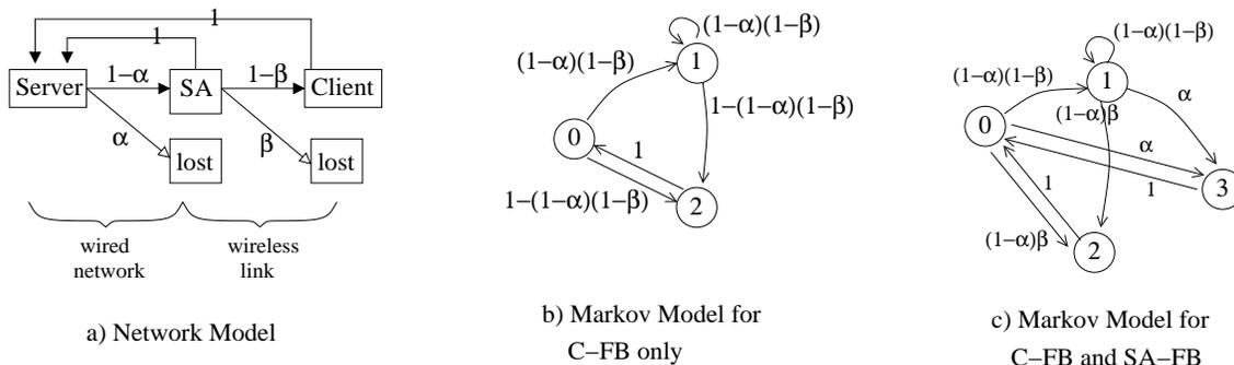
Fig. 2. Abstract Network Model and Markov Chains for Feedback Systems
