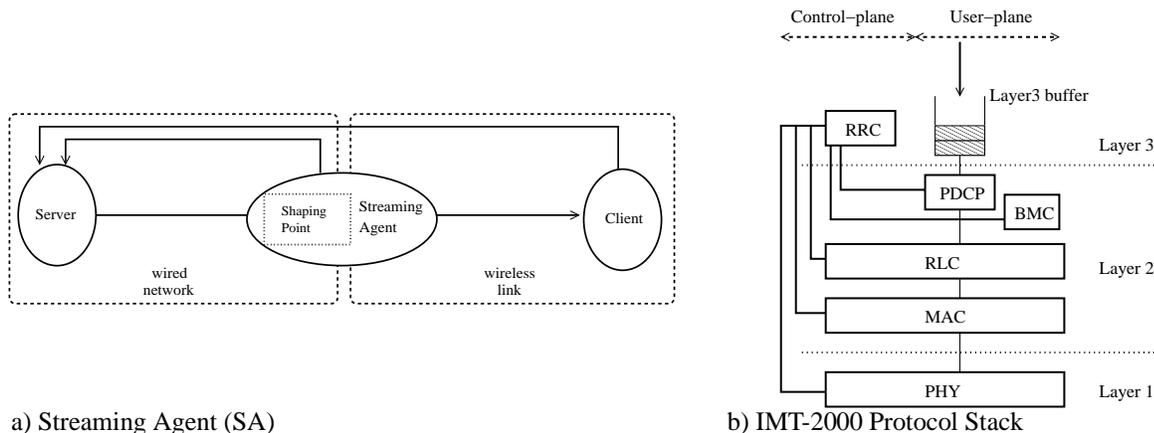
Fig. 1. Streaming Agent and 3G link-layer Protocol Stack
