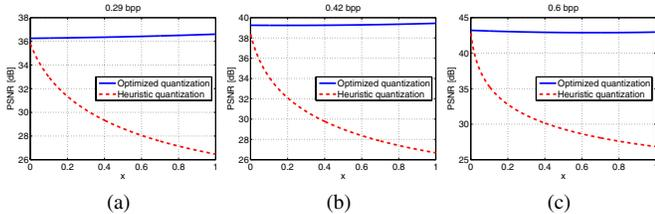
**Fig. 2.** Distortion  $D(Q, x)$  for  $x \in [0, 1]$  using the heuristic quantizer  $Q_h$  (red) and optimal quantizer  $Q^*$  (blue). The graphs are shown for the total bit rates (a) 0.29 bpp, (b) 0.42 bpp and (c) 0.60 bpp. The maximal distortion is significantly reduced in all cases when the optimized quantization is applied.
