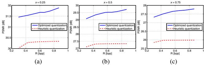
**Fig. 3.** The RD performance of view synthesis at 3 viewpoints (a)  $x = 0.25$ , (b)  $x = 0.5$  and (c)  $x = 0.75$ . The optimized quantization results in an improved quality of the synthesized views than the heuristic quantization.
