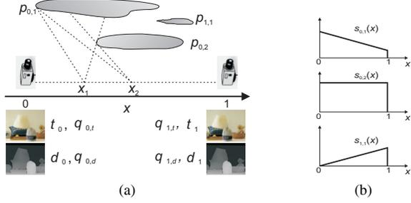
**Fig. 1.** (a) The coding problem setup. The shown examples of the captured texture and depth images are taken from the data set `Midd2` [10]. (b) The sizes of the visible portions of 3 patches are approximated by linear functions of the synthesis viewpoint location  $x$ .
