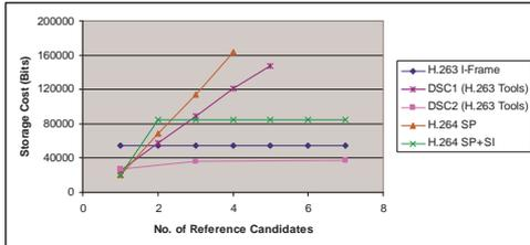
**Fig. 3.** Storage costs comparison (Akko&Kayo). The x-axis represents the number of decoding paths, and the y-axis represents the average number of bits to encode a picture  $F_{i,j}$ , e.g.,  $B_{DSC1}$  for DSC1.
