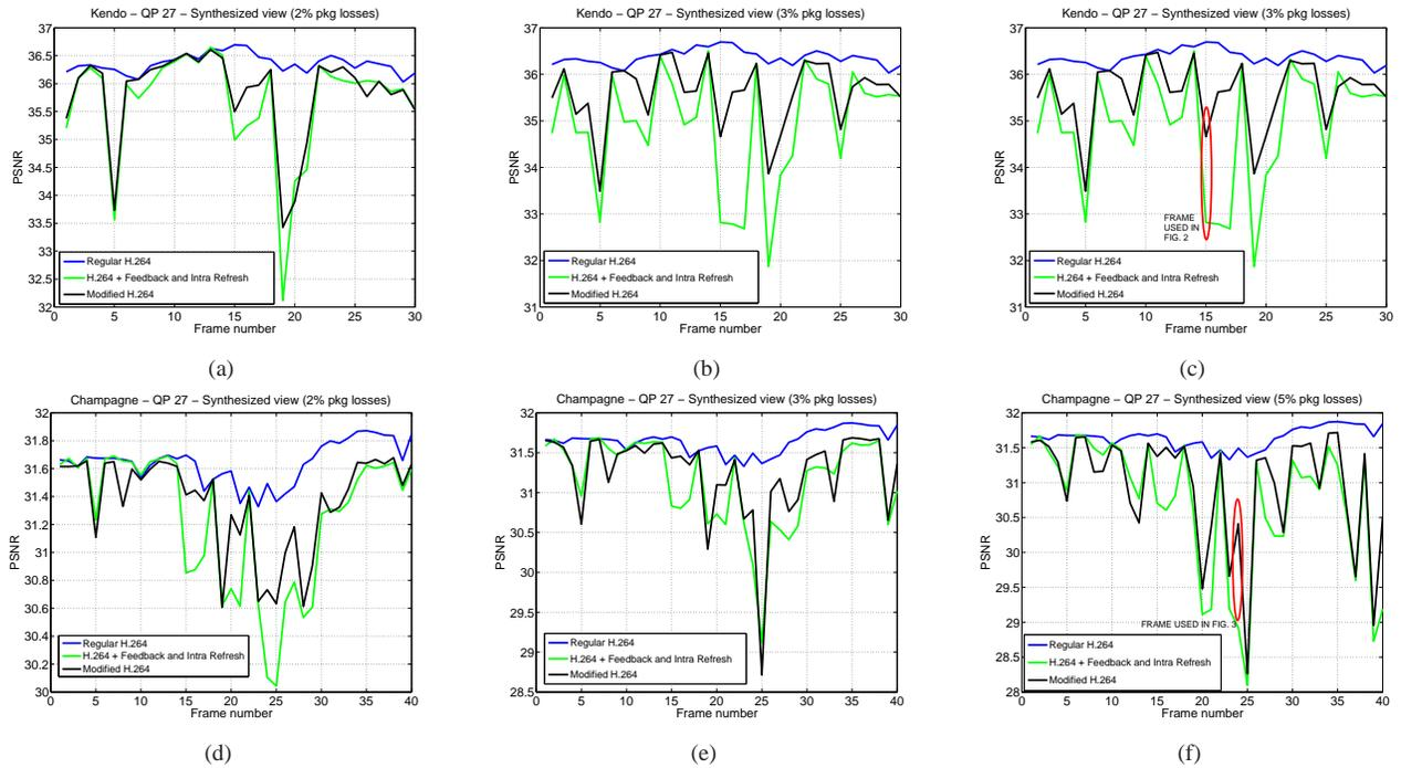
**Fig. 1.** PSNR vs Frame plots for Kendo at  $1024 \times 768$  pixels (top row) and Champagne at  $1280 \times 960$  (bottom row). The bitrates for Kendo are 6.6 Mbps for *Conventional H.264*, and 9.0 Mbps for both “*Conventional H.264 + Feedback and Intra Refresh*” and *Modified H.264*. For Champagne, the bitrates are 5.0 Mbps and 8.0 Mbps, respectively.
