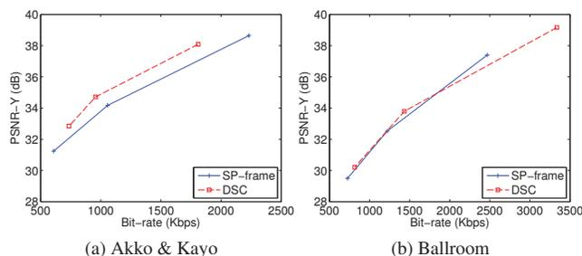
**Fig. 7.** Expected transmission cost, with switching probability  $\alpha$  equal to 0.2. DSC tends to perform better when view switching is more likely. See [2] for comparison with other settings of  $\alpha$ .
