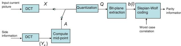
Fig. 3. DSC frame encoding.
