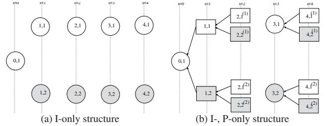
**Fig. 2.** Examples of frame structures for IMVS for two views (white and grey for view 1 and 2) and  $M = 1$ . Circles, rectangles are I- and P- frames, respectively.
