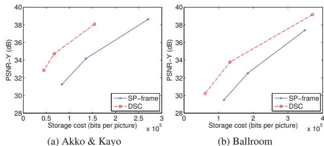
**Fig. 6.** Average storage cost per picture, at different reconstruction quality. In DSC, different reconstruction quality can be achieved by varying the quantization parameters for the intermediate P-frames and the targets.
