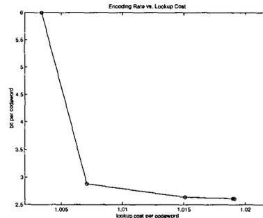
Figure 11: Tradeoff between Bit Rate and Decoding Time
