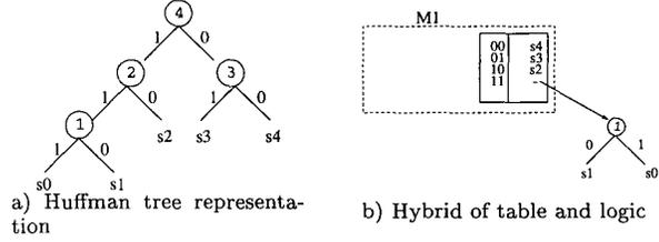
Figure 5: Example of VLC Decoding
