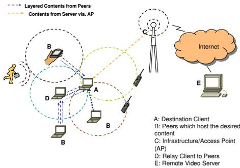
Fig. 1. Joint Server/Peer Video Streaming over Wireless Network
