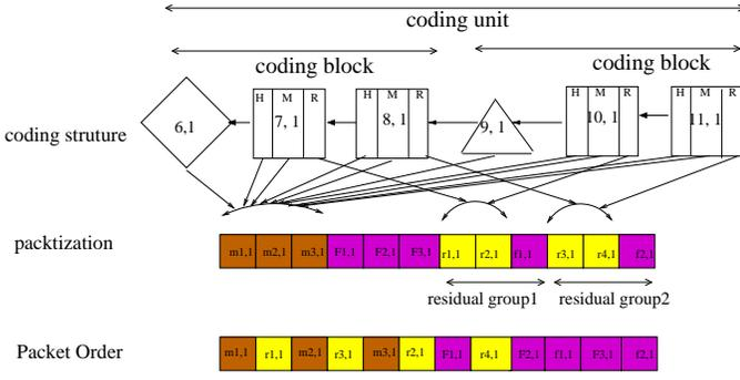
Fig. 4. The three stages of the transmission scheme: i) encoding of captured images into frames in coding structure, ii) packetization of encoded bits into IP packets, and iii) ordering of generated packets for transmission. Motion, residual and FEC packets are indicated by red, yellow and blue, respectively.
