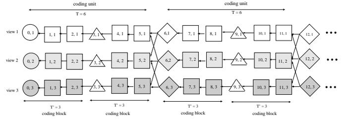
Fig. 3. Example of proposed coding structure for  $M = 3$  views and coding block size  $T' = 3$ , coding unit size  $T = 6$ . Circles, squares, triangles and diamonds are I-, P-, DE-DSC and MP-DSC frames. Each frame  $F_{i,v}$  is labeled by its time index  $i$  and view  $v$ .
