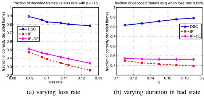
Fig. 5. Comparison of fraction of decoded frames for different coding structures: (a) buffer time, (b) varying average duration in bad state in DE model while WWAN loss rate is fixed at 0.0969.
