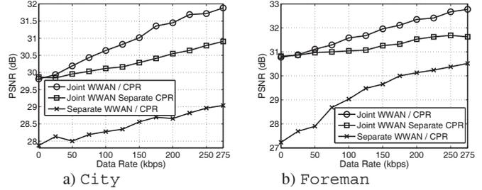
Fig. 2. Joint WWAN-CPR optimization versus joint WWAN separate CPR, and separate WWAN-CPR optimizations.
