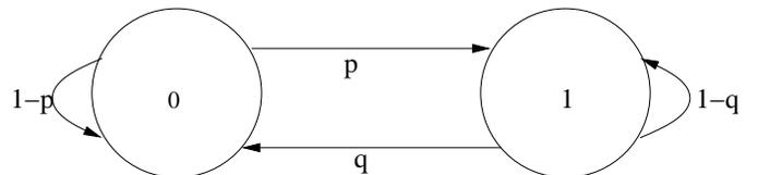
Fig. 2. Gilbert-Elliott loss model: The channel transitions between its two states (good - 0 and bad - 1) with probabilities  $p$  and  $q$ . The packet loss probabilities in good and bad states are  $g$  and  $b$ , respectively.
