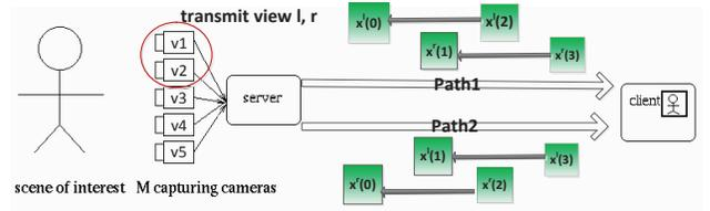
Fig. 1. Overview of the multi-path free-viewpoint video transmission system. Multiple descriptions are constructed for transmission over two disjoint paths.
