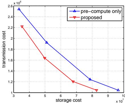
Figure 2. Tradeoff between storage and transmission with  $p_{pb} = 0.5$ .
