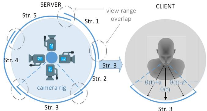
**Fig. 1.** Interactive VR video streaming system using 5 pre-encoded streams with overlapping view ranges. Corresponding to user's head rotation angle  $\theta(t)$  and FoV  $[\theta(t) - a, \theta(t) + a]$  at time  $t$ , stream 3 is selected and transmitted.
