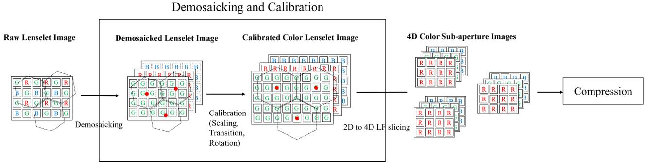
Fig. 1: Conventional coding scheme for light field image. The demosaicing and calibration processes are applied before compression.
