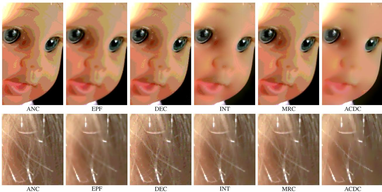
Fig. 9: Simulation of displaying the output images in 6-bit experiment ( $b = 6$ ) on HBD monitor (cropped regions of `im4`).
