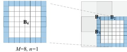
Fig. 6: Illustration of boundary pixels and boundary condition. Suppose the gray blocks have been processed,  $\mathbf{B}_4$  is the current  $8 \times 8$  block with 28 boundary pixels (marked in blue).
