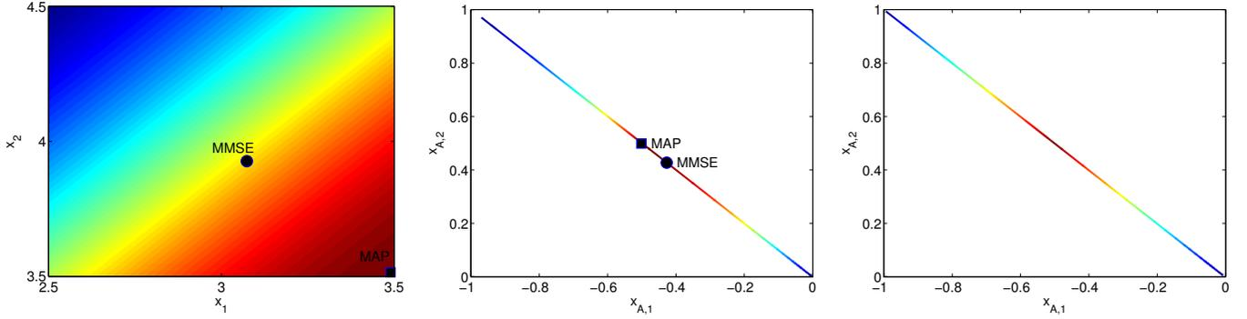
(a) Posterior PDF  $f(\mathbf{x}|\mathbf{y})$  in direct MAP (9). Likelihood function (4) defines a square feasible space where the MAP solution is at the corner. (b) Posterior PDF of AC signal  $f(\mathbf{x}_A|\mathbf{y})$  in MAP AC estimation (23). Note MAP solution is close to MMSE solution. (c) Likelihood function of AC signal (20) in MAP AC estimation (23). Feasible space of AC signal (21) is a line segment.
