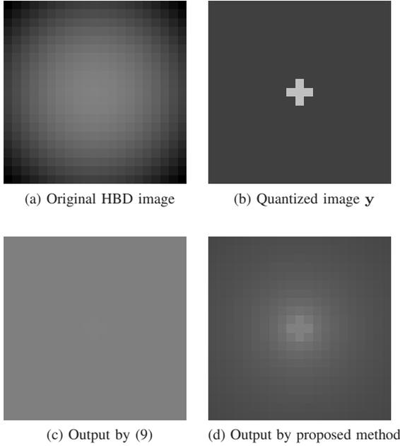
Fig. 4: Example showing direct MAP estimation leads to a DC output (c) with large MSE, while proposed two-step approach outputs a smooth signal (d) with smaller MSE.
