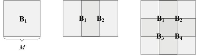
Fig. 2: Illustration of block arrangement. We use  $M \times M$  half-overlapped blocks to reduce artefacts due to block-based processing. From left to right: one block, two overlapped blocks, four overlapped blocks. Note that the boundary pixels of a block are the inner pixels of other blocks.
