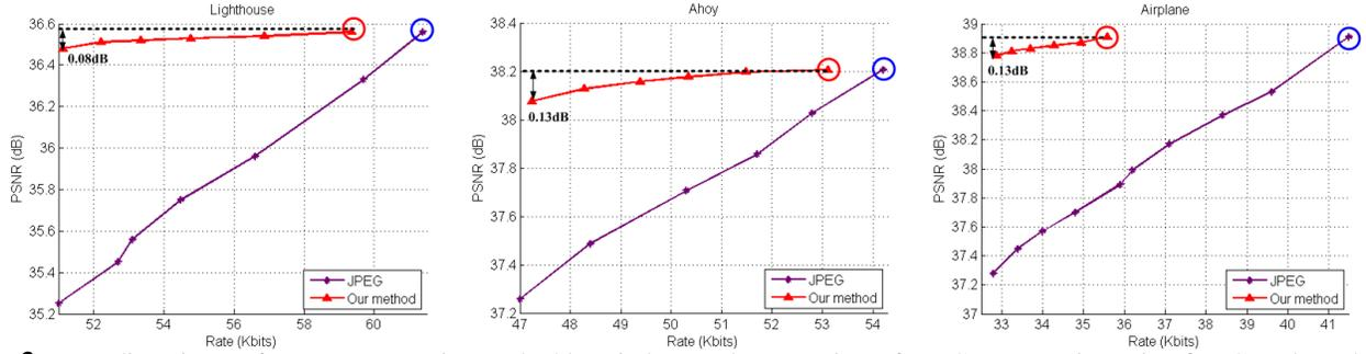
**Fig. 3.** Rate-distortion performance comparison. The blue circles are the RD points of JPEG compression using fine QF. The red circles represent the RD points of signal fidelity reconstruction by our method. The red and blue circles have the same PSNR values, but red ones use less bits.
