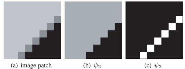
**Fig. 2.** An example of the *hard boundary* and *borders* of smooth and transition regions in a GPWS signal: (a) GPWS image patch; (b) the corresponding second eigenvector of the graph Laplacian, using which the hard boundary can be identified; (c) the corresponding third eigenvector, using which the borders of the smooth / transition regions can be identified.
