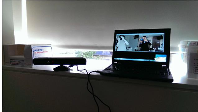
**Fig. 1:** Depth video capturing system at a sleep clinic: a MS Kinect camera is attached to a laptop computer. Example depth and infrared captured images are shown on the screen.
