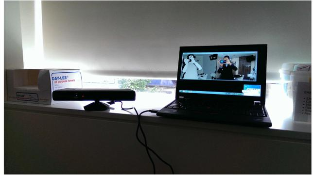
**Fig. 1:** Depth video capturing system at a sleep clinic: a MS Kinect camera is attached to a laptop computer. Example depth and infrared captured images are shown on the screen.
