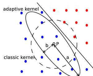
Figure 3. Illustration of adaptive kernel on a pixel patch with stripes of blue and red pixels: an ellipse is elongated along a direction perpendicular to the principal gradient, so that only similar pixels are selected for pixel interpolation.
