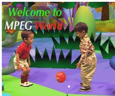
Fig. 2. An unreliable eye gaze tracker often produces noisy observations. In this example, a viewer has focused on the red ball in this frame 220 of MPEG test sequence kids , but an eye tracker reports gaze location marked by the 5 \times 5 white square.
