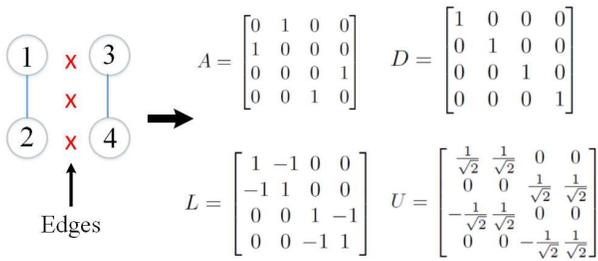
Fig. 2. An example of constructing GBT from a  $2 \times 2$  pixel block. The vertical edges separate pixel 1 and 2 from pixel 3 and 4 and a graph is constructed by connecting pixels on each side of the edges. The corresponding adjacency matrix  $\mathbf{A}$ , degree matrix  $\mathbf{D}$ , Laplacian matrix  $\mathbf{L}$  as well as the computed GBT  $\mathbf{U}$  are shown on the right.
