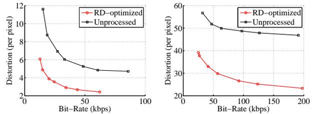
**Fig. 2:** Distortion-rate curve of the RD-optimized surface and the unprocessed surface comparing against ML surface for *Lovebird1* (left) and *Balloons* (right).
