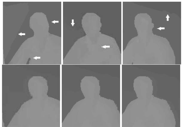
**Fig. 3:** Comparing unprocessed with ML depth maps for *Lovebird1* (for clarity in visual presentation, all pixel values are increased by 80). From top to bottom: unprocessed depth maps at views 4,6,8; ML solution at views 4, 6, 8.
