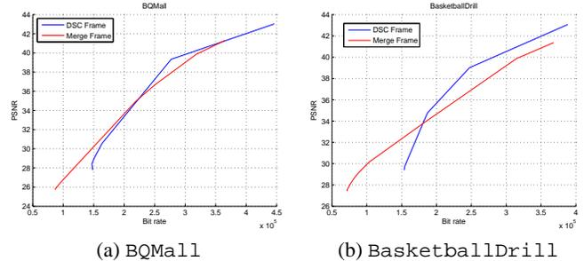
Fig. 4. PSNR versus encoding rate comparing proposed merge frame with DSC frame in [6] for sequences `BQMall` and `BasketballDrill`.
