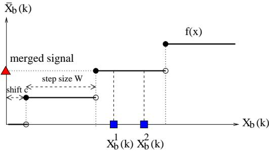
**Fig. 1.** Given the side information  $X_b^1(k)$  and  $X_b^2(k)$  corresponding to the  $k$ -th coefficient of block  $b$ , a pwc function  $f(x)$  maps them to the same  $\bar{X}_b(k)$  if they fall on the same step. Only step size  $W$  and shift  $c$  are needed to specify pwc function  $f(x)$ , which we encode for each coefficient.
