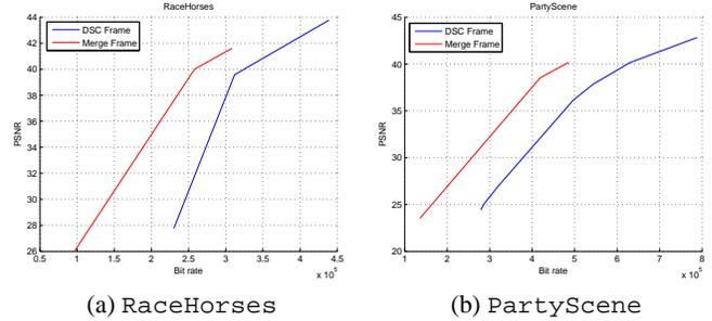
Fig. 3. PSNR versus encoding rate comparing proposed merge frame with DSC frame in [6] for sequences `RaceHorses` and `PartyScene`.
