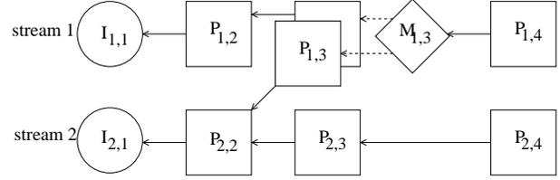
**Fig. 2.** Example of stream-switching from one pre-encoded stream to another using merge frame. SI frames ( $P_{1,3}$ ’s) are first constructed using different predictors. Then merge frame  $M_{1,3}$  is encoded using the two SI frames. I-, P- and merge frames are represented as circles, squares and diamonds.
