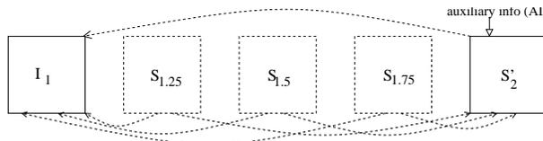
**Fig. 2.** Example of rate-complexity tradeoff for high-spec devices. Virtual views 1.25, 1.5, 1.75 are synthesized at client using views 1 and 2 as reference (shown as dashed lines). Reference view 2 is reconstructed via view synthesis from reference view 1, with the help of transmitted AI to inpaint disoccluded regions to complete the image.
