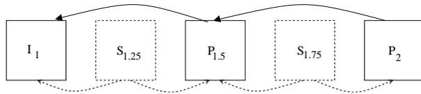
**Fig. 1.** Example of rate-complexity tradeoff for low-spec devices. In addition to reference views 1 and 2, virtual view 1.5 is rendered and encoded as a P-frame  $P_{1.5}$  at server, so that only virtual views 1.25 and 1.75 are synthesized at client (each using two nearby encoded frames as reference, shown as dashed lines), reducing overall complexity.
