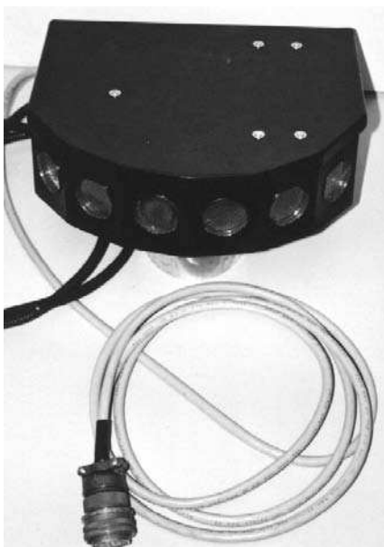
Figure 3.14: Outside SONAR Array. Note the six Polaroid 600 series transducers and the grey cable used for micro-controller signals.
