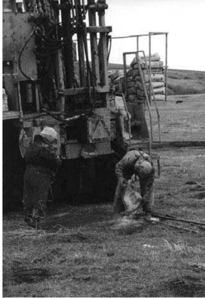
Figure A.3: Sealing seismic explosives behind rig (Pincher Creek, AB; 1999).
