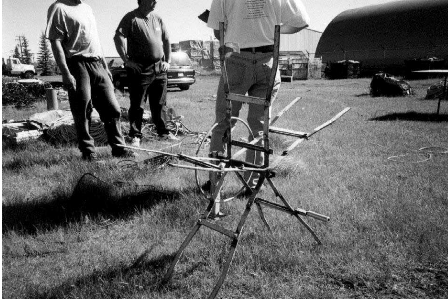
Figure A.7: A seismic cable spooler (Photo: Ryan Chladny; Airdrie, AB; 1999)
