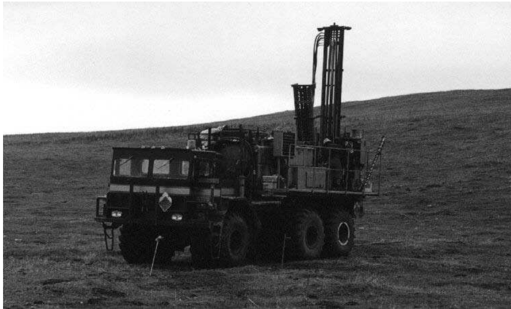
Figure A.2: Seismic explosives drilling rig (Pincher Creek, AB; 1999).
