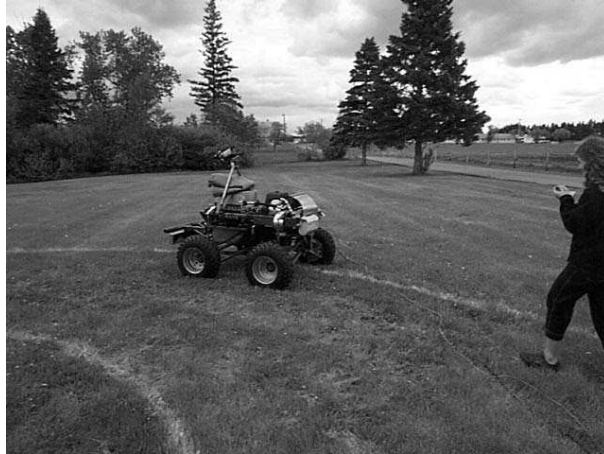
Figure 2.1: Demonstration of the Polar Bear robot driving autonomously using a video camera to follow a white line (another possible application apart from those discussed in this thesis). (University of Alberta Experimental Farm, Edmonton, AB; 1998)
