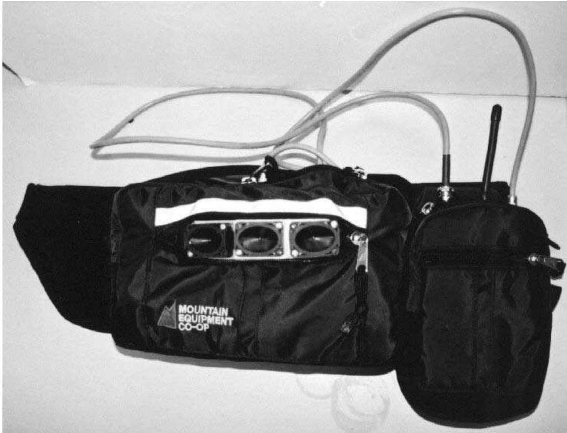
Figure 3.16: The Complete Pursuit Pack. Note the three Polaroid 9000 series transducers in the centre and the Freewave DGR-115 frequency hopping spread-spectrum radio in the pouch on the right.
