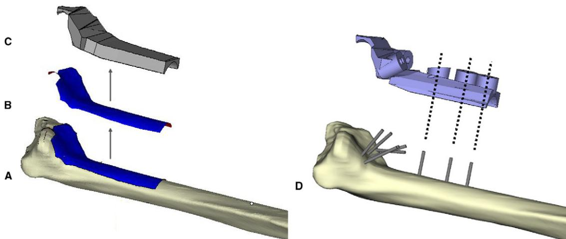
**FIGURE 3:** Creation of patient-specific instrument guide. **A** Selection of the registration surface. **B** Extracting the mirror image of the registration surface. **C** Integration of the mirror bone image into the patient-specific template. **D** Integration of the instrument guidance into the template with respect to the planned screw location.
