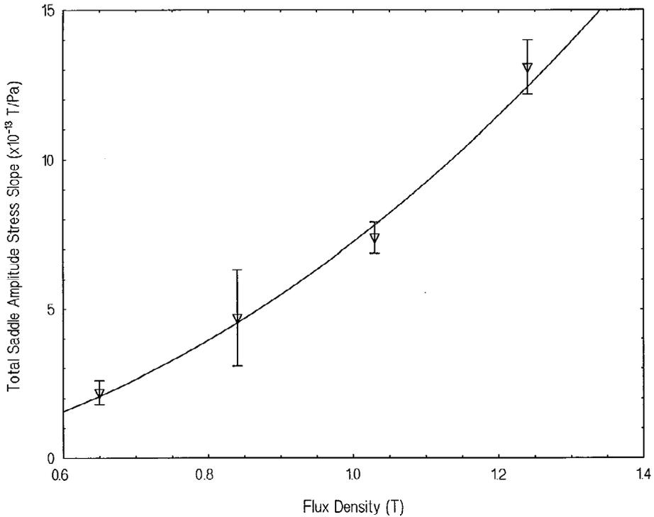
**Fig. 8.** Sum of positive and negative saddle amplitude stress slopes plotted as a function of pipe wall flux density for the after-cycle ( $\nabla$ ) in the composite beam ( $B = 1.24$  T). The solid curve is simply a line to guide the eye.
