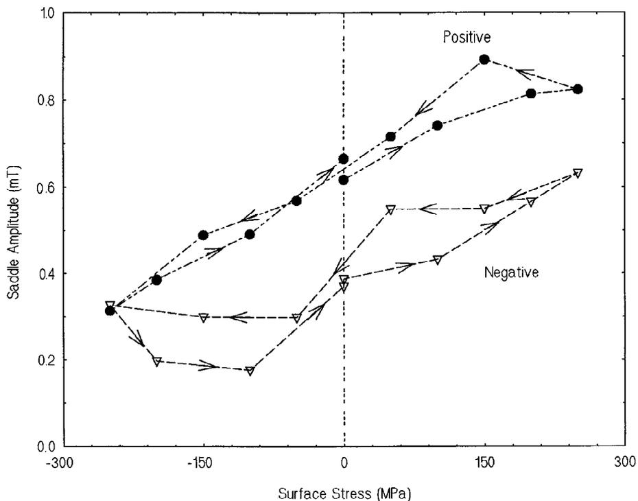
**Fig. 4.** Positive (●) and negative (▽) saddle amplitudes as functions of surface stress using the semi-circular pipeline apparatus with a field of 1.54 T during the normal cycle are plotted for the 13-mm ball-milled 50% defect.
