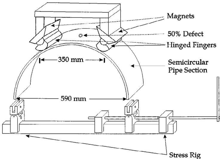
**Fig. 1.** The semicircular pipe section and bending stress rig for the production of surface stress in semicircular sections of pipe steel.
