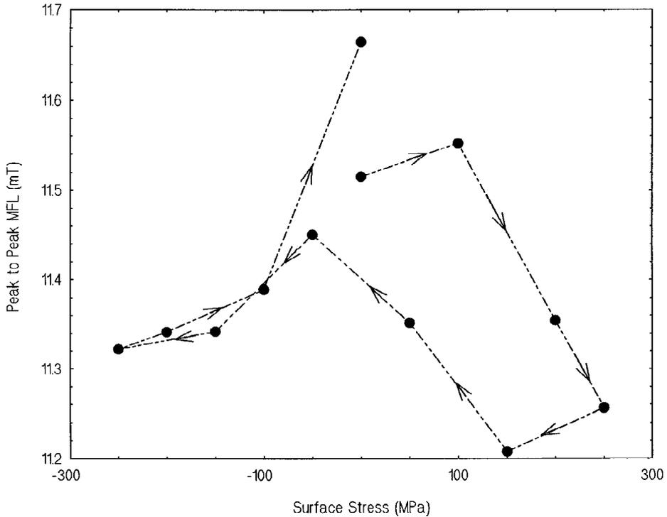
**Fig. 3.** Peak-to-peak MFL signal from the near side as a function of surface stress in the normal cycle for a 13-mm-diameter ball-milled 50% defect on the semicircular pipe section under hoop-bending stress with an applied pipe wall flux density of 1.54 Tesla at 0 MPa.
