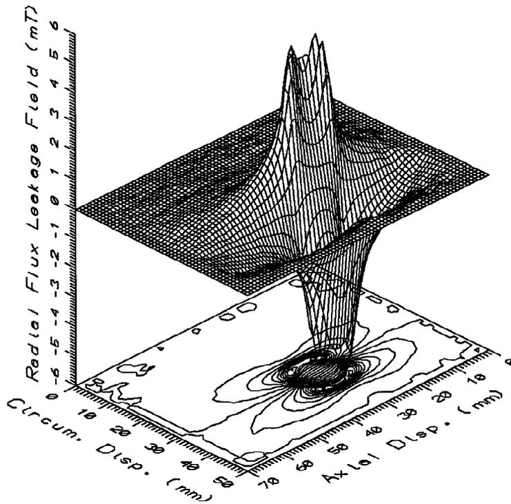
**Fig. 2.** (a) Surface and contour plots of the radial magnetic flux leakage from the near side of a 13-mm-diameter ball-milled 50% defect in the semicircular pipe section under a tensile stress of 250 MPa during a normal cycle.
