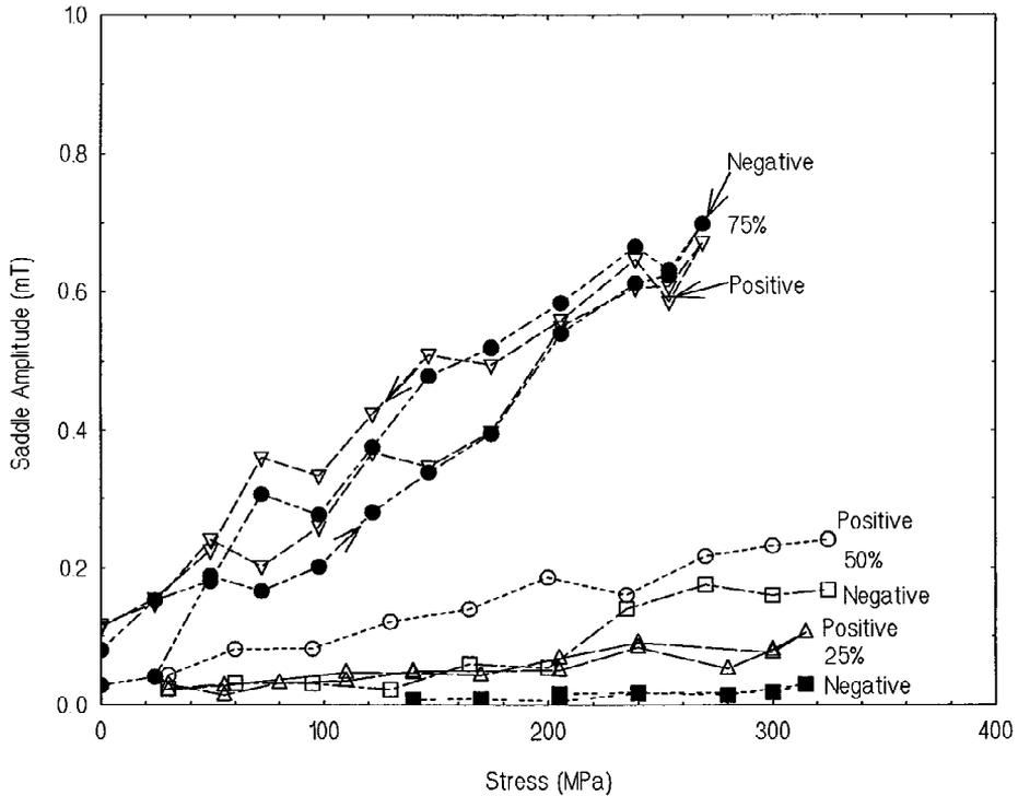
**Fig. 5.** Saddle amplitudes as a function of stress in the composite beam apparatus from 13-mm ball-milled defects in a field of 1.24 T in the normal cycle are plotted for the 25% defect for the positive ( $\Delta$ ) and negative ( $\blacksquare$ ), for the 50% defect for the positive ( $\circ$ ) and negative ( $\square$ ), and for the 75% defect for the positive ( $\nabla$ ) and negative ( $\bullet$ ) saddle amplitudes.
