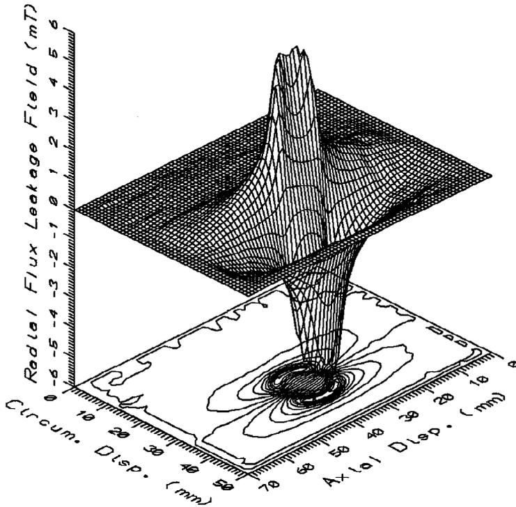
**Fig. 2.** (b) Surface and contour plots of the radial magnetic flux leakage from the near side of a 13-mm-diameter ball-milled pit in the semicircular pipe section under compressive stress at 250 MPa during a normal cycle.
