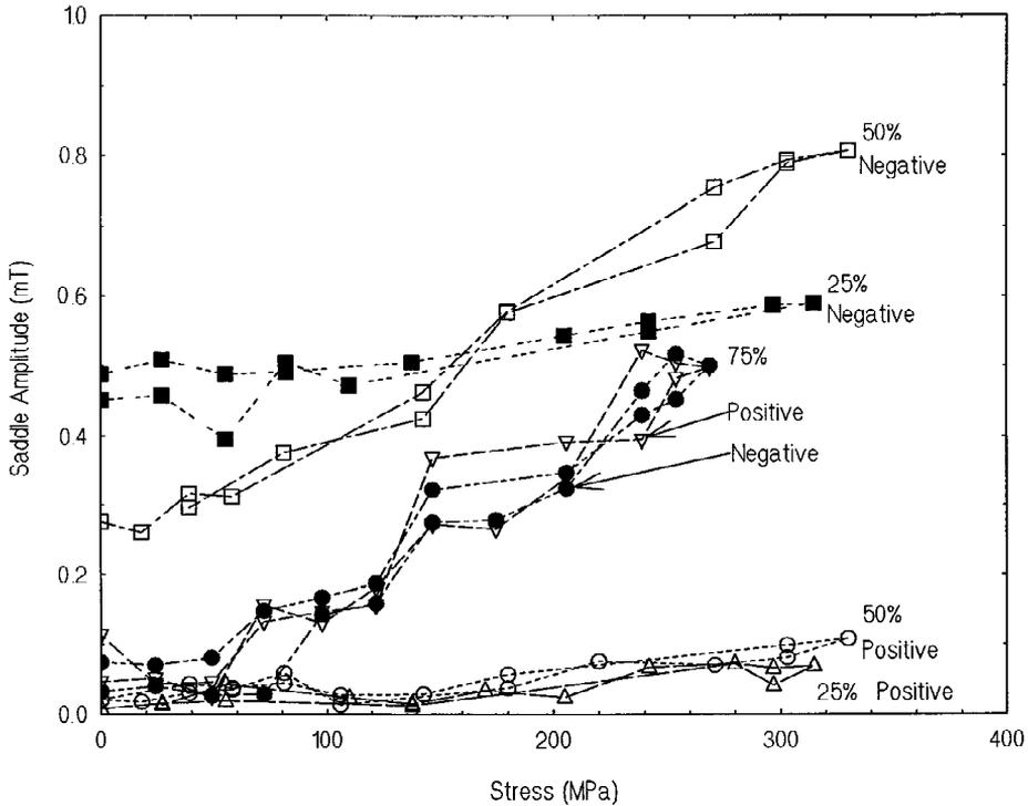
**Fig. 6.** Saddle amplitudes as a function of stress in the composite beam apparatus from 13-mm ball-milled defects in a field of 1.24 T in the after-cycle are plotted for the 25% defect for the positive ( $\Delta$ ) and negative ( $\blacksquare$ ), for the 50% defect for the positive ( $\circ$ ) and negative ( $\square$ ), and for the 75% defect for the positive ( $\nabla$ ) and negative ( $\bullet$ ) saddle amplitudes.
