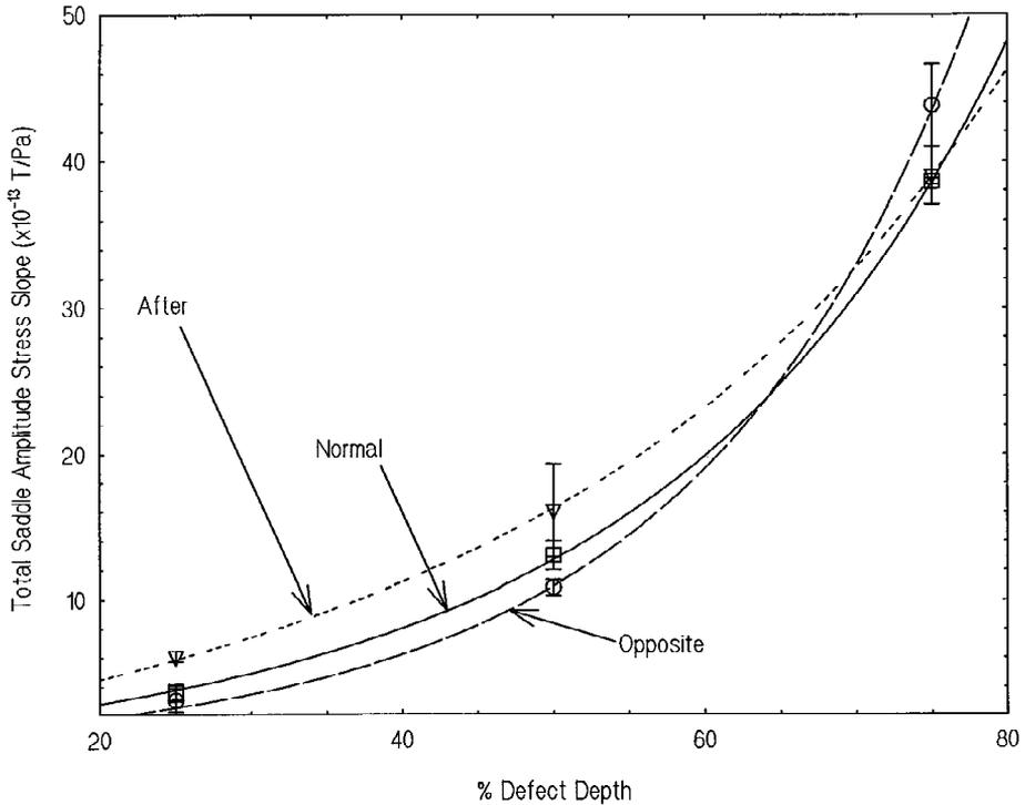
**Fig. 7.** The sum of positive and negative saddle amplitude stress slopes plotted as a function of % defect depth for the normal cycle (□), after-cycle, (▽) and opposite cycle (○) in the composite beam ( $B = 1.24 T$ ). The solid and dashed curves are lines to guide the eye.
