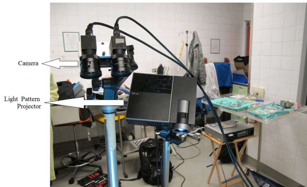
Figure 1: Original Stereo and Groundtruth Acquisition System.
