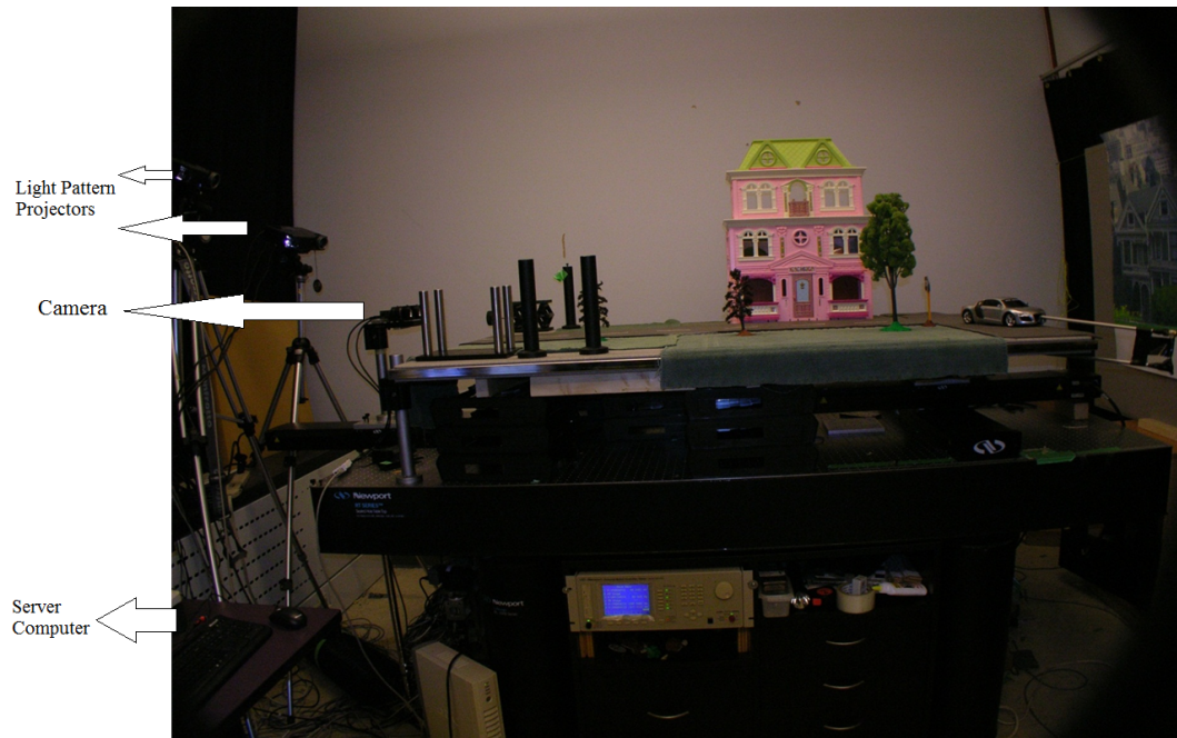
Figure 1: Original Stereo and Groundtruth Acquisition System.
