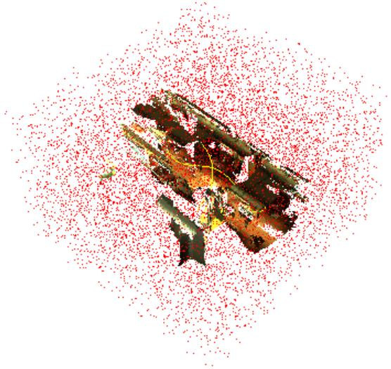
Figure 3.11: A uniform distribution of particles across the position search space. This example uses 10,000 particles for the search space.
