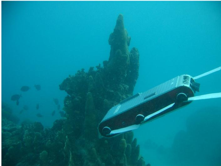
Figure 1.3: The 6DOF amphibious underwater robot AQUA [29]. Pose estimation algorithms for such a device must consider the device’s ability to assume nearly any orientation in 3D space.
