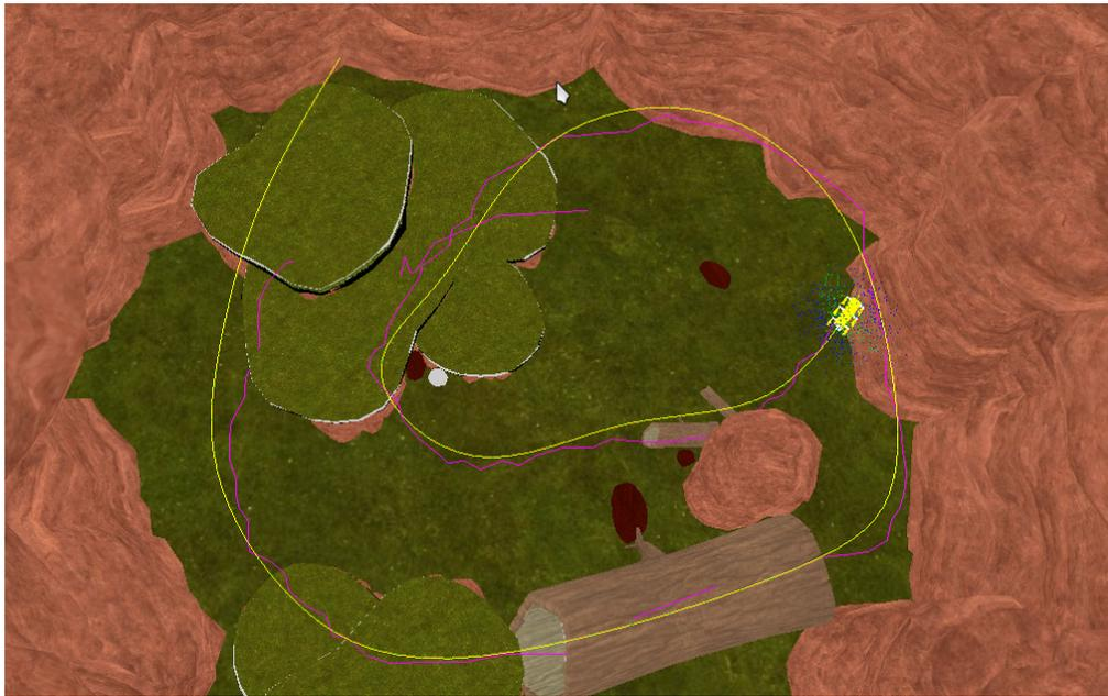
(a) Mini Level, particle filter with EKF, 750 particles.  $\sim 30$  msec per update.
