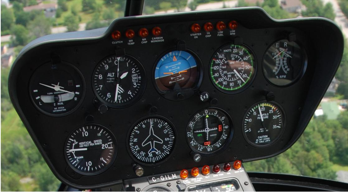
Figure 3.1: Instrument panel on a helicopter showing, among other things gyro, heading and altitude dials. Aircraft pilots rely on these instruments to maintain safe flight, when personal instincts may be unreliable.
