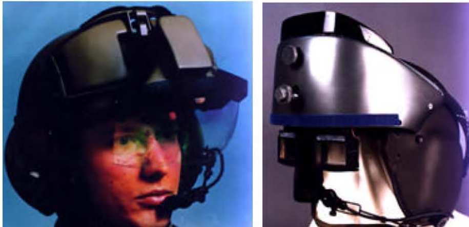
Figure 6 - Two optical see-through HMDs, made by Hughes Electronics, images from [5].
