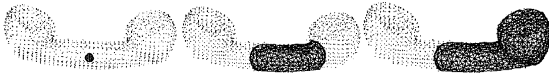
Figure 4.10. Dynamic inflating balloon. The algorithm starts with an icosahedron inside the object (left), then this balloon is growing (centre) until the mesh arrive to the surface of the object, stopping there but growing in other directions (right). (Source: Chen & Medioni, 1995 )
