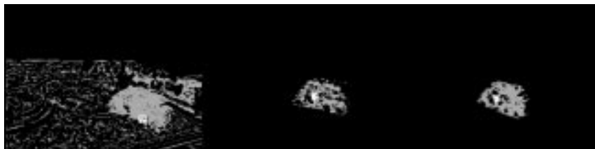
Segment corresponding to the turning truck with seed region highlighted.
