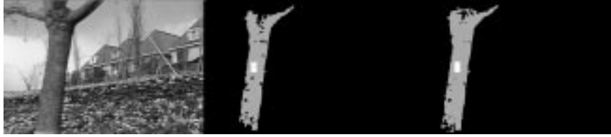
Figure 3.8: Flower Garden image sequence. The moving tree in the foreground of the flower garden is segmented out by tracking a seed region on the tree trunk. The optimized \vec{\sigma}_o parameters are: \sigma_n = 1.28 , \sigma_a = 0.23 , \sigma_u = 0.128 , \sigma_v = 0.359 , \sigma_l = 0.0078 , \sigma_f = 0.45 .
