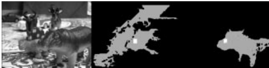
Frame 15 and its output from tracker using default \vec{\sigma}_{def} and optimized \vec{\sigma}_o .
