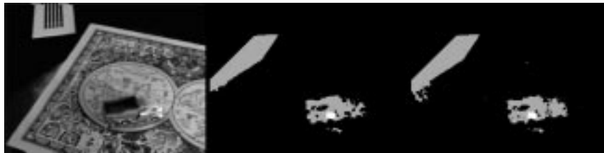
Frame 1 and its output from tracker using default \vec{\sigma}_{def} and optimized \vec{\sigma}_o .
