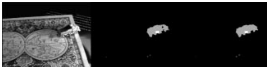
Frame 41 and its output from tracker using default \vec{\sigma}_{def} and optimized \vec{\sigma}_o .
