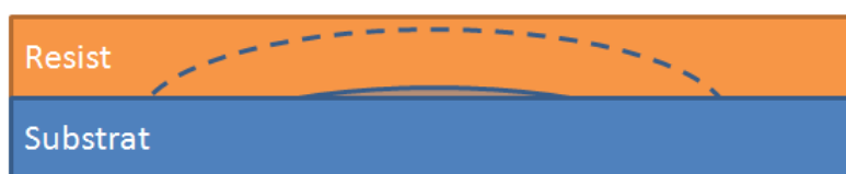
Figure 24 : Upper part of the microlens too weakly insulated = too low value.
