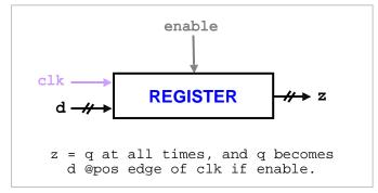
As all sequential components, a **register** has an internal state, denoted by  $\mathbf{q}$ , and it is made up of  $\mathbf{n}$  bits, where  $\mathbf{n}$  is a parameter set upon instantiation. The output  $\mathbf{z}$  is equal to  $\mathbf{q}$  at all times; i.e. you can always *read* the content of a register. In order to *write* (i.e. store) a value in the register, supply the value through  $\mathbf{d}$ , set **enable** to 1, and then wait until the **clk** input rises from 0 to 1.
