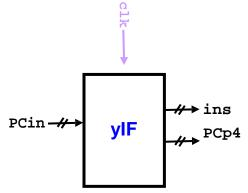
Given a memory address **PCin**, this circuit fetches from memory the instruction **ins** stored at that address and makes it available. The circuit also computes and outputs PCp4 = PCin + 4 in anticipation of fetching the physically-following instruction.
