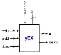
This unit performs the operation specified via the op signal. We assume the same 3bit operation codes used by the ALU. The operands are rd1 and either rd2 or imm depending on whether ALUSrc is 0 or 1.
