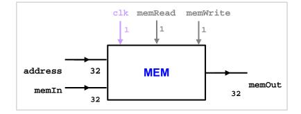
This sequential component is made up of many 32-bit words. In order to read a word, set its address on address and set memRead. After some delay, the word's content will become stable on memOut. To write, set the data to be written on memIn, set the destination address on address, and set memWrite. The data will be written on the destination at the next positive edge of clk.
