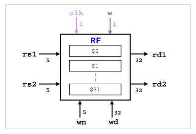
In order to read the contents of two registers, we supply their register numbers thru rs1 and rs2 (5 bits each). After some delay, the corresponding contents of these two registers will become stable on rd1 and rd2. In order to store a 32-bit value in some register, we supply it on wd and supply the 5-bit register number on wn. The value will be written on the positive edge of clk if and only if w=1. Hence, w is in fact an enabler. Note that register \$0 is read-only and its value is 0.
