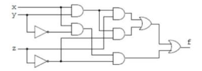
• The function f(x, y, z) simplifies to  $x(y + \overline{z})$ .
